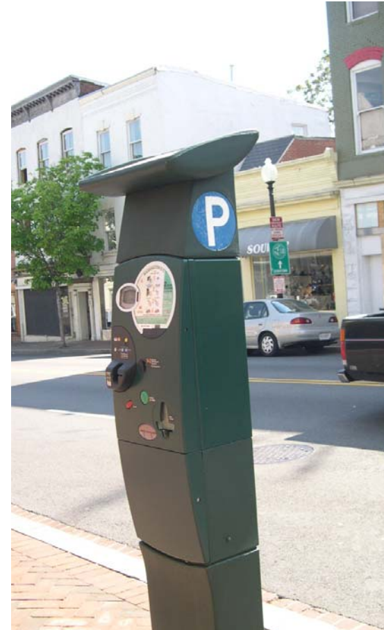
SOLAR POWERED MULTISPACE PARKING METER ALLOWS FOR MORE FLEXIBLE MANAGEMENT AND CREDIT/DEBIT CARD PAYMENT
