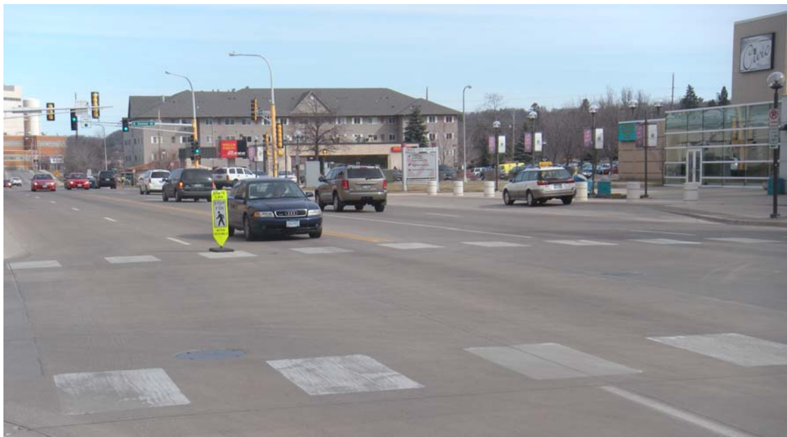
WIDE STREET RIGHTS-OF-WAY WITH NO CENTER REFUGE CREATE INTIMIDATING CROSSINGS FOR PEDESTRIANS (CIVIC CENTER DRIVE)
