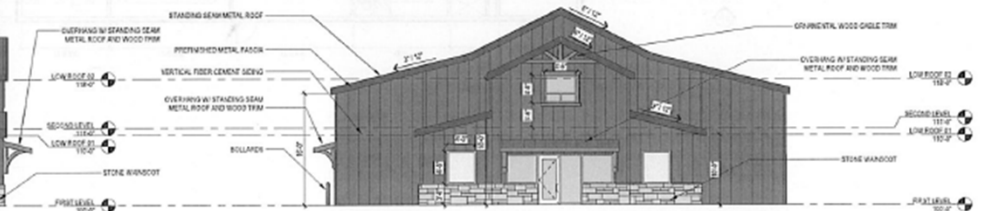
ELEVATION - SHOP, NORTH SCALE: 1/8" = 1'-0"
