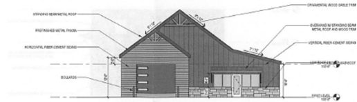
ELEVATION - SINGLE TENANT, NORTH SCALE: 1/8" = 1'-0"
