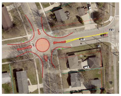
Mini roundabout that forces drivers to slow down to navigate the roadway.
