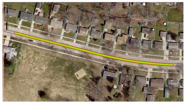
Concrete curb and gutter median approximately 725' x 20' with landscaping that does not allow on street parking.
