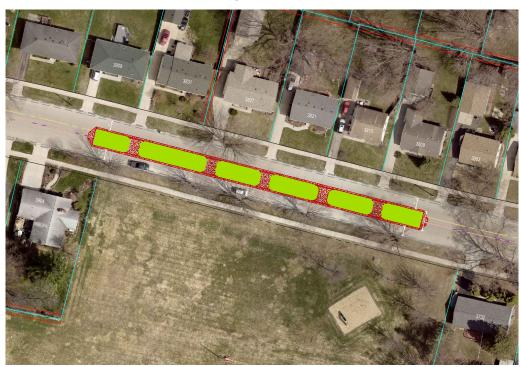
Concrete curb and gutter median approximately 340' x 20' with landscaping and driveway egresses that does not allow on street parking.
