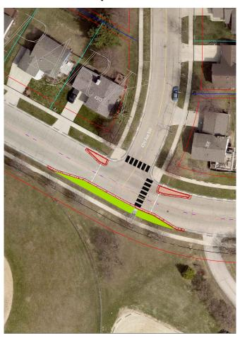
Concrete curb and gutter bump outs and road choker to narrow the road width and force drivers to slow down to navigate the roadway.
