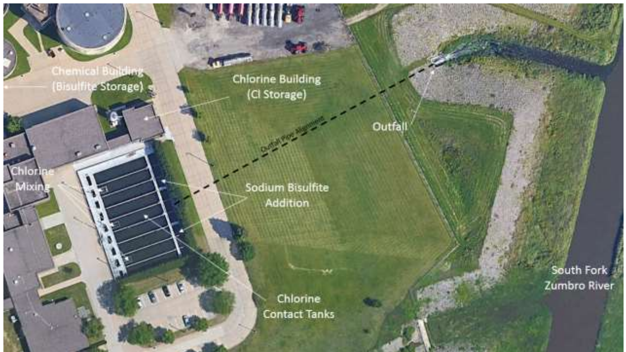
Figure 1-1. WRP disinfection and outfall site layout
