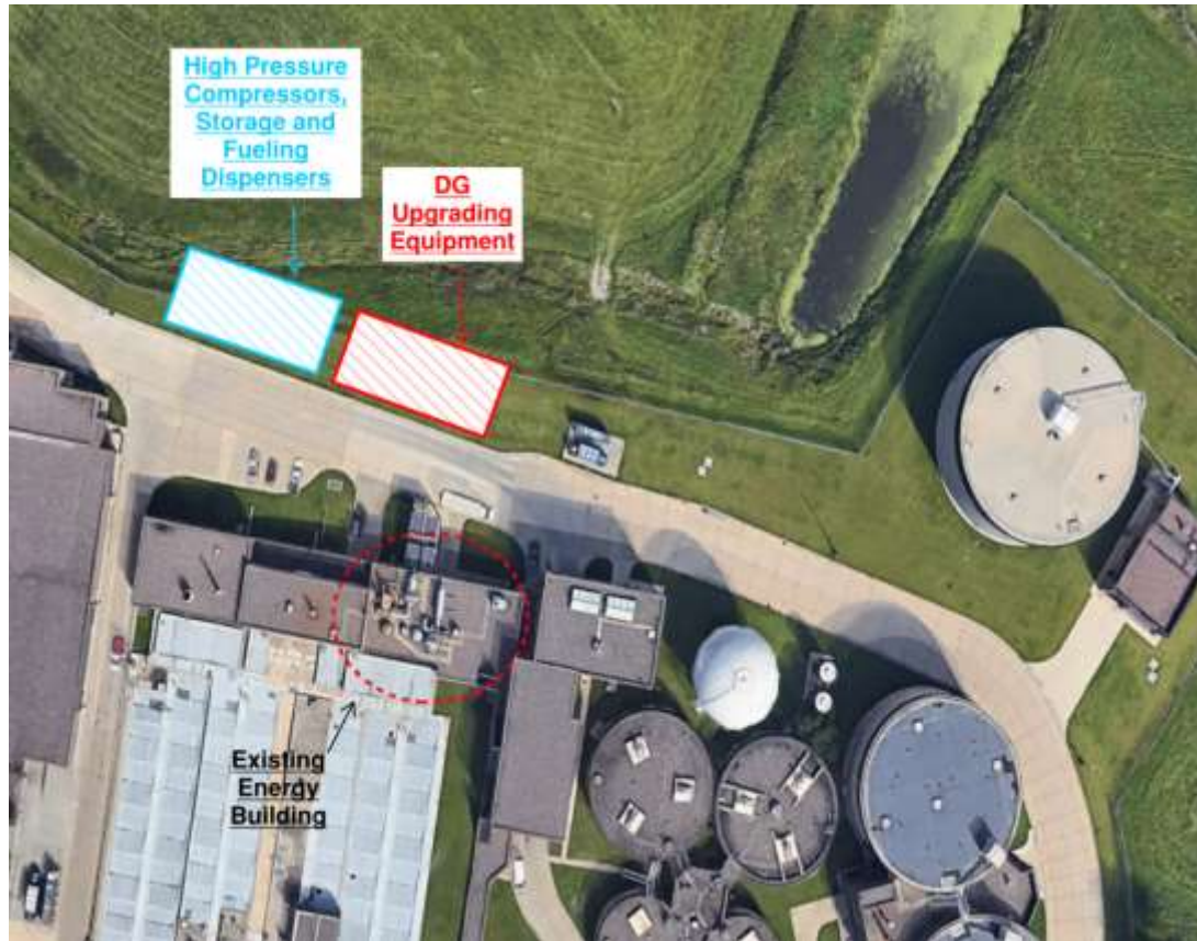
Figure 2-12. On-site vehicle fueling site layout
