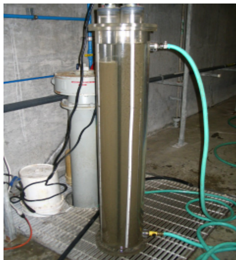
Figure 2-2. Settling Column Used for Batch Settling Tests
