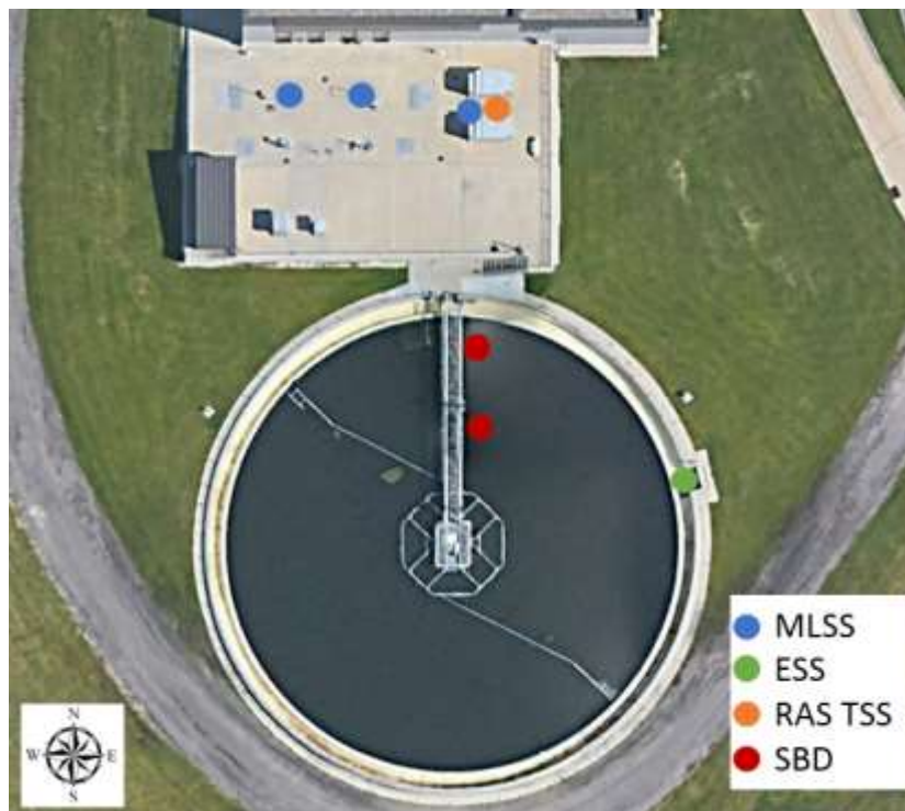
Figure 2-3. Final Clarifier 5 stress test sample locations
