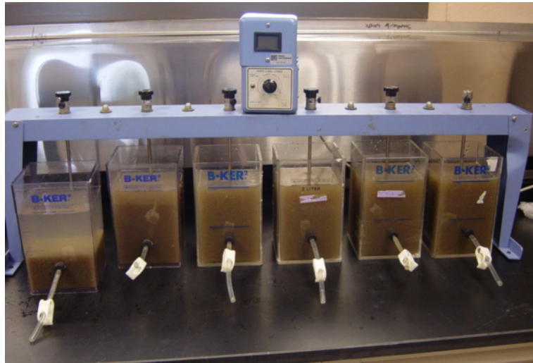
Figure 2-3. Flocculation Jar Test Apparatus
