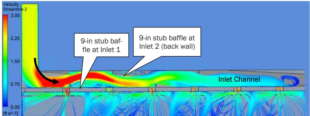
Figure ES-6. Primary Clarifier 2 recommended inlet channel stub baffle configuration
