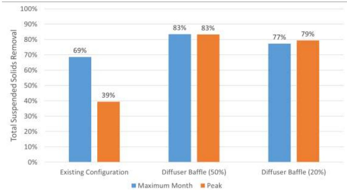
**Figure 3-9. Predicted TSS removal for various diffuser baffle porosities at maximum month and peak conditions**
