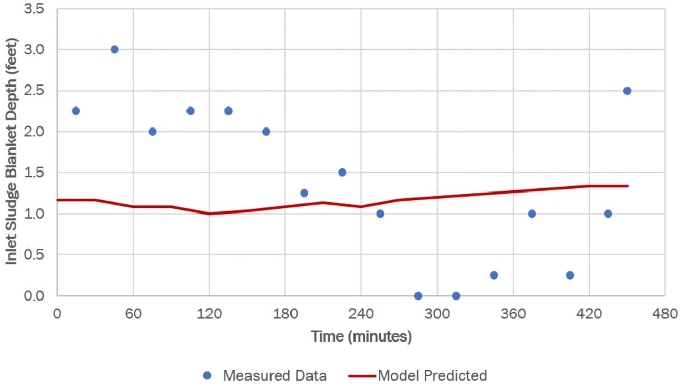
Figure 2-8. Primary Clarifier 2 measured and predicted SBD at inlet end
