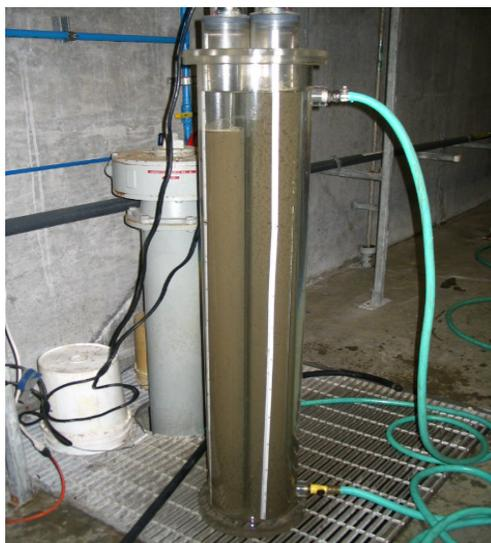
Figure 2-2. Settling Column Used for Batch Settling Tests
