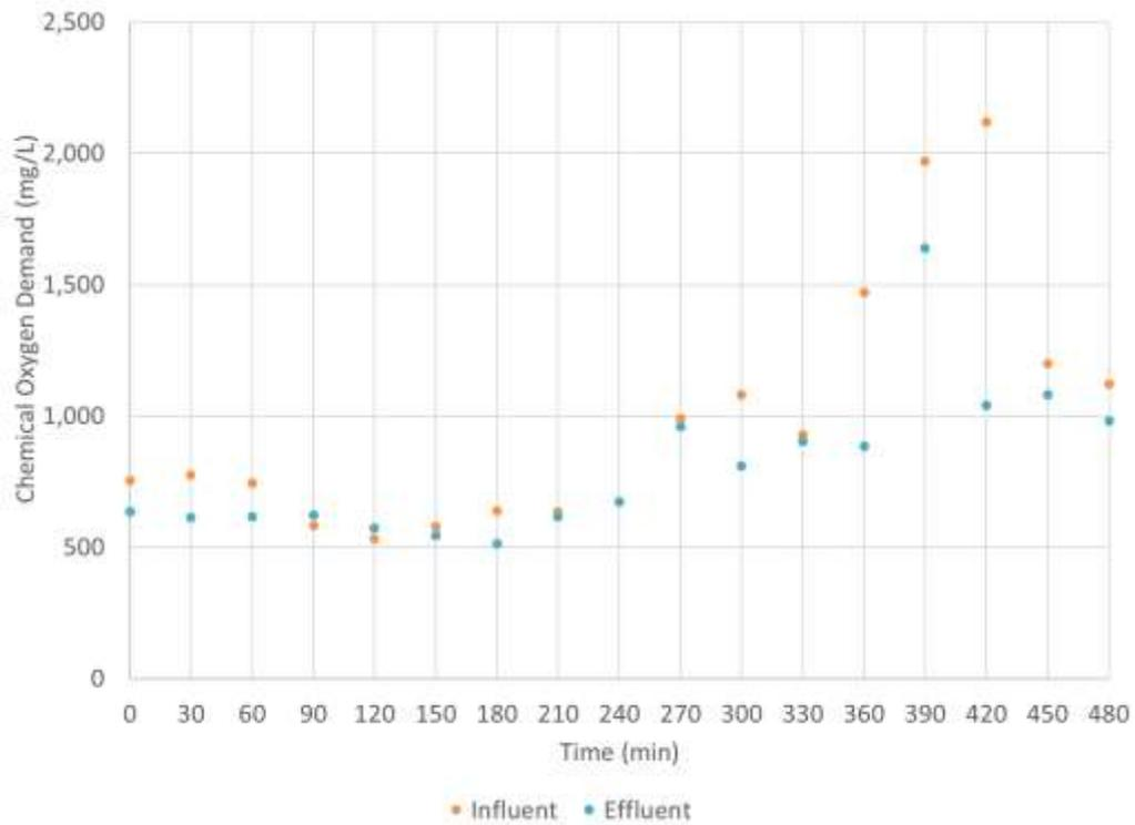
Figure 5-1. Stress test Primary Clarifier 2 influent and effluent total COD
