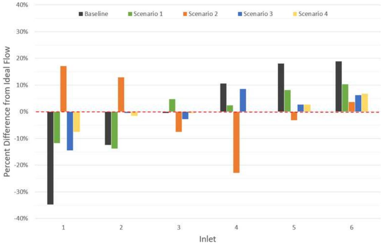
**Figure 4-4. Primary Clarifier 2 predicted inlet channel flow distribution**
