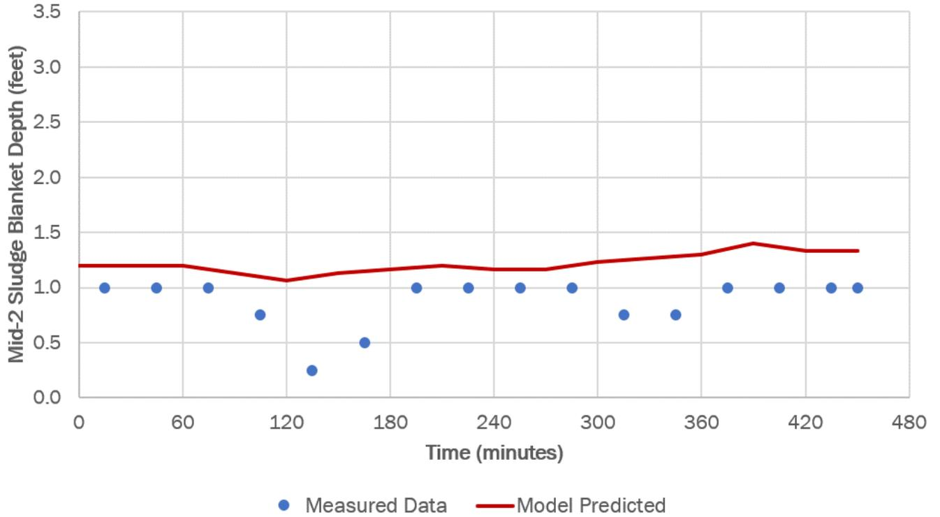
Figure 2-10. Primary Clarifier 2 measured and predicted SBD at Middle-2 location
