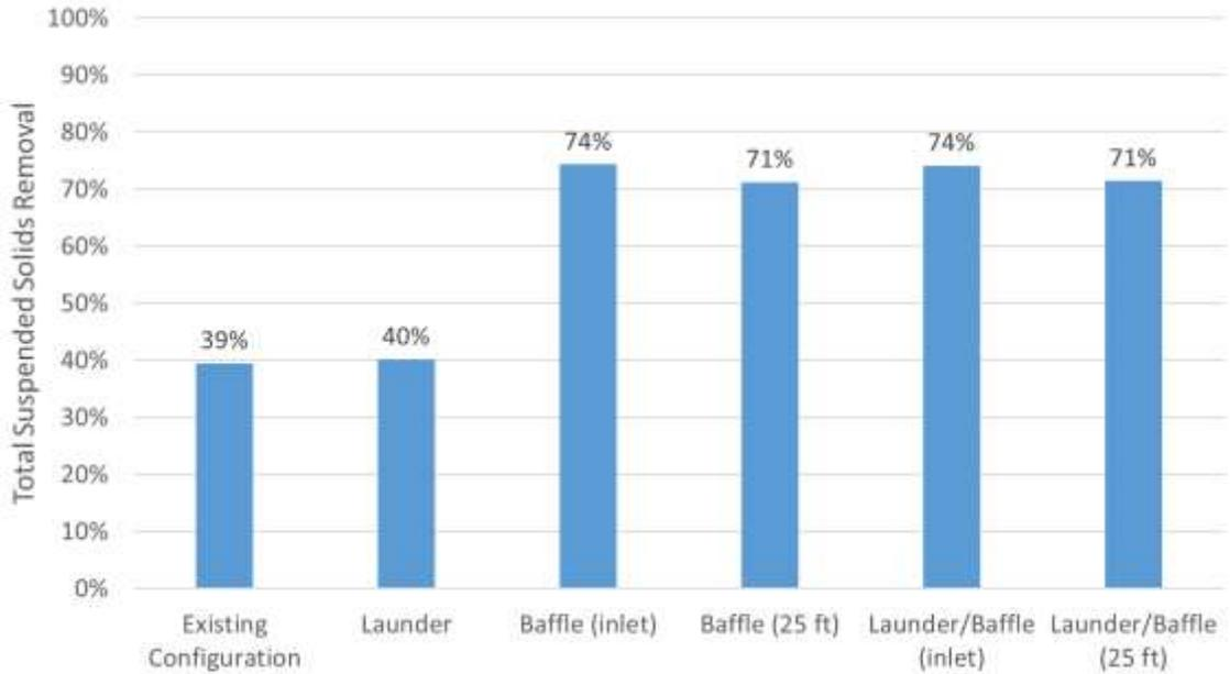
**Figure 3-7. Predicted TSS removal for combined enhancements or alone**
