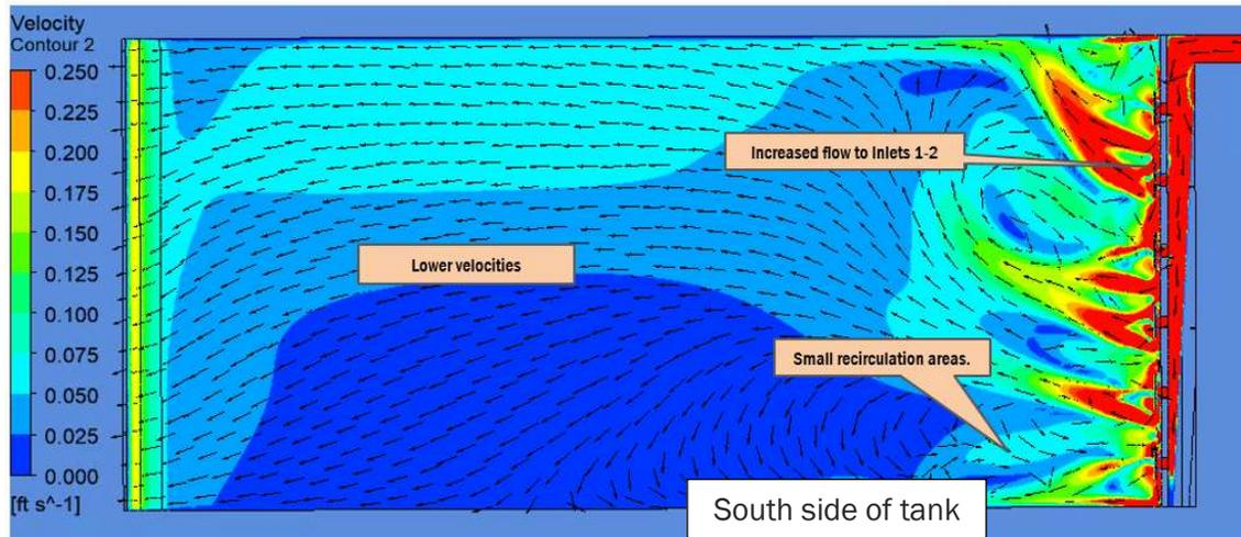
Figure ES-7. Primary Clarifier 2 diffuser plate Alternative 2 stream lines - plan view (includes inlet stub baffles)
