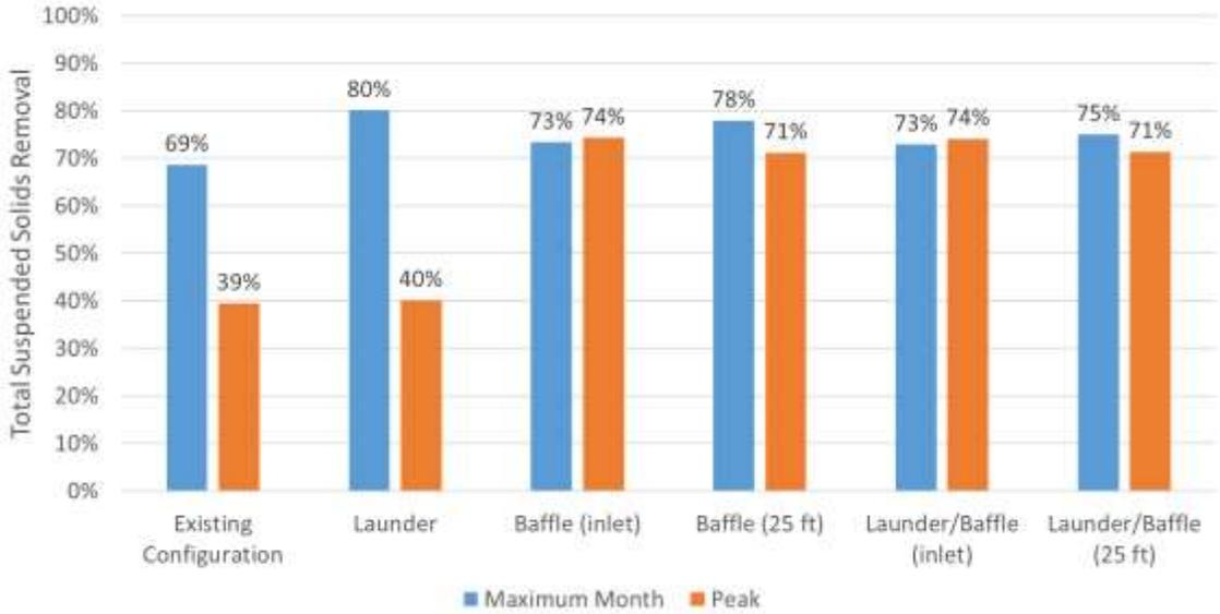
**Figure ES-2. Relative comparison of predicted primary clarifier TSS removal for combined enhancements or alone**
