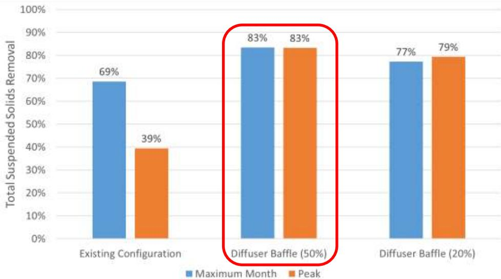
**Figure ES-3. Predicted TSS removal for various diffuser baffle porosities at maximum month and peak conditions**
