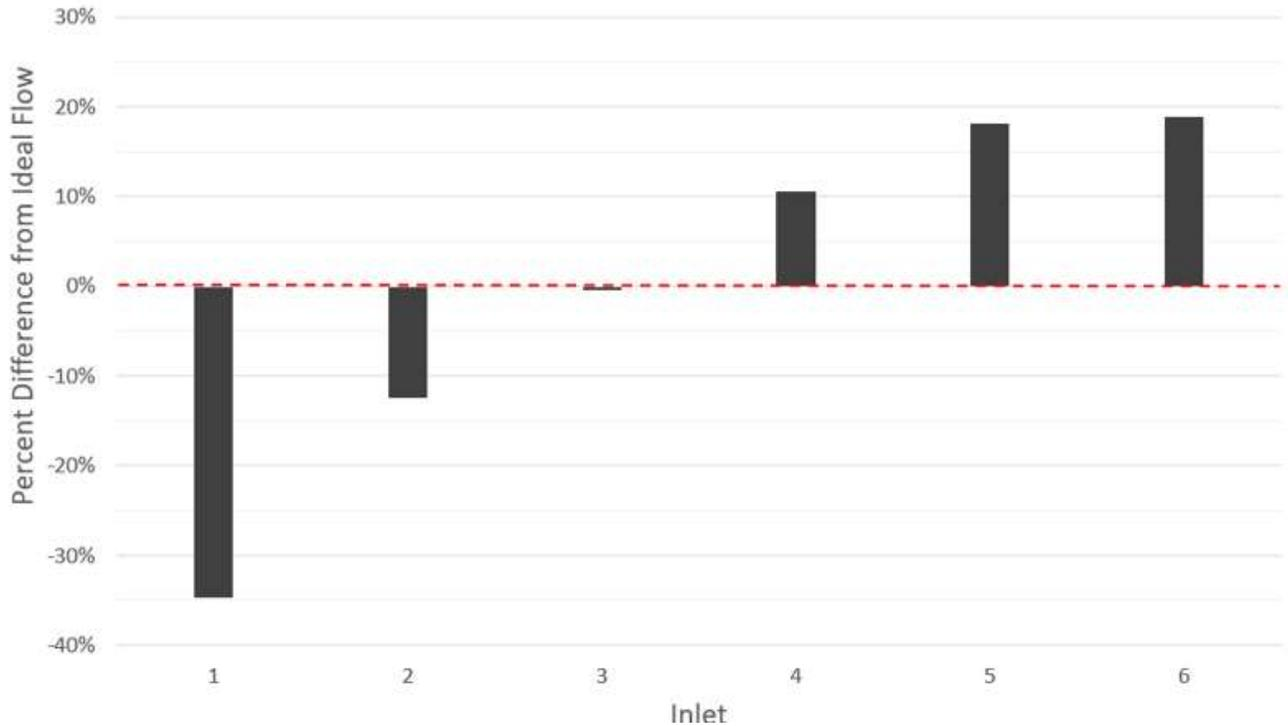
Figure 4-2. Primary Clarifier 2 predicted inlet port flow distribution
