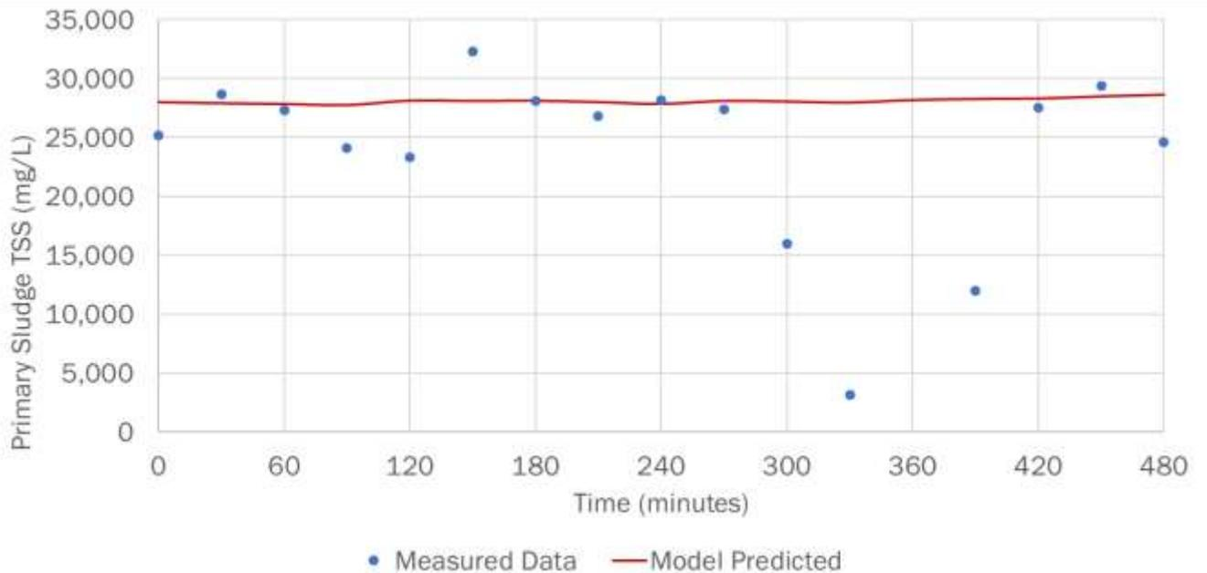
Figure 2-7. Primary Clarifier 2 measured and predicted primary sludge TSS
