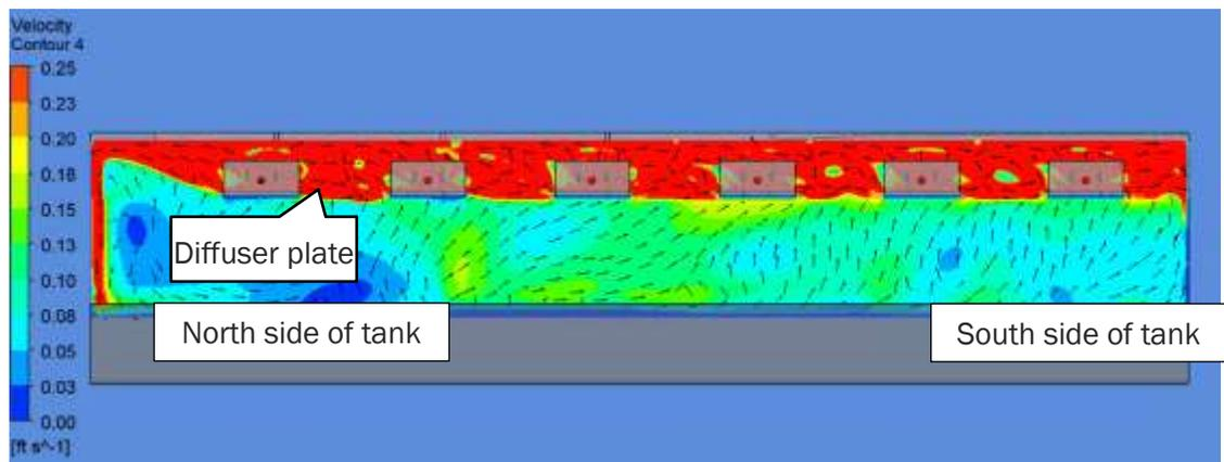
Figure 4-15. Primary Clarifier 2 diffuser plate Alternative 2 stream lines – section view (includes inlet stub baffles)
