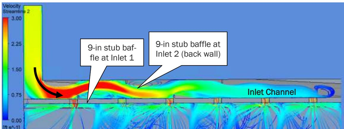
Figure 4-3. Primary Clarifier 2 inlet channel stub baffle configuration – Scenario 4
