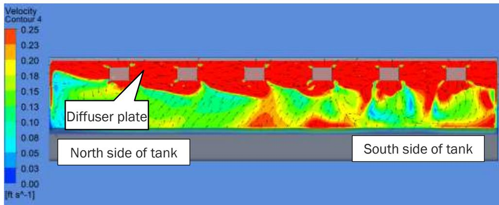
Figure 4-10. Primary Clarifier 2 existing diffuser plates – section view
