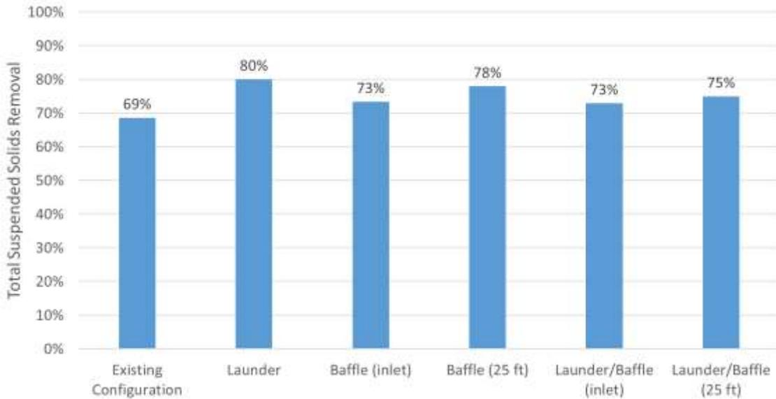
**Figure 3-6. Predicted TSS removal for combined enhancements or alone**
