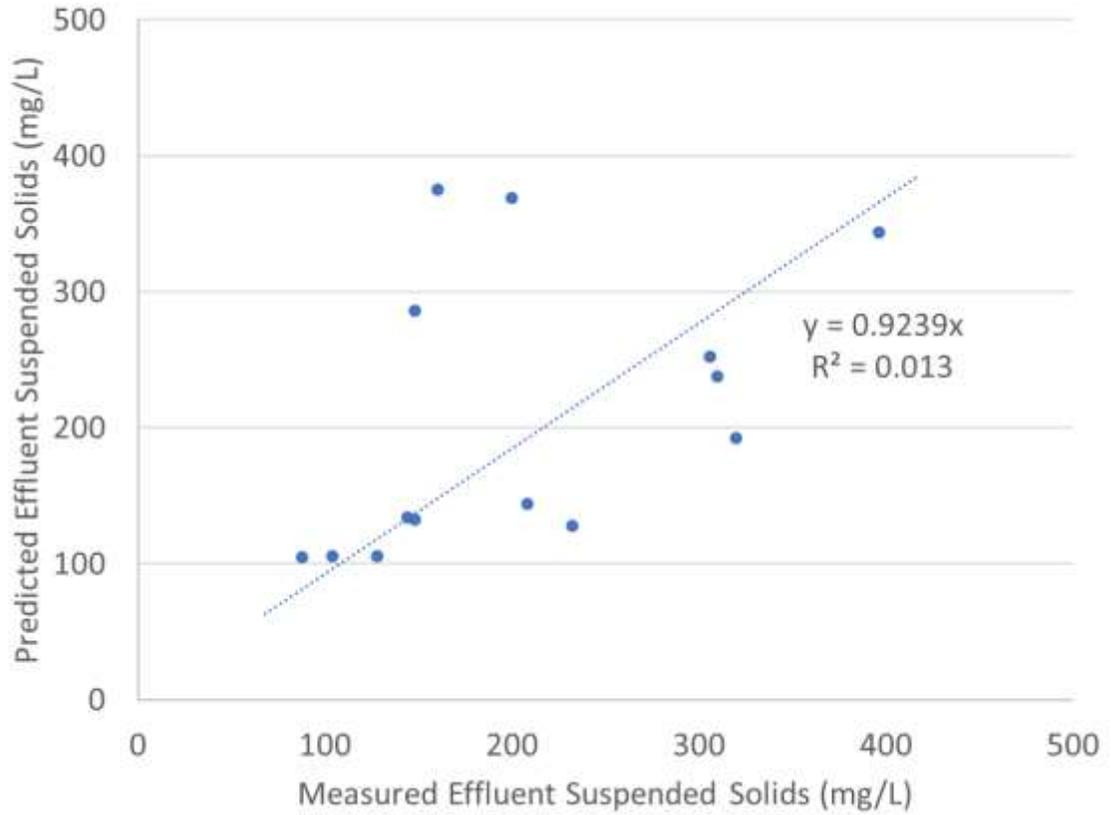
Figure 2-6. Primary Clarifier 2 measured and predicted PE TSS correlation
