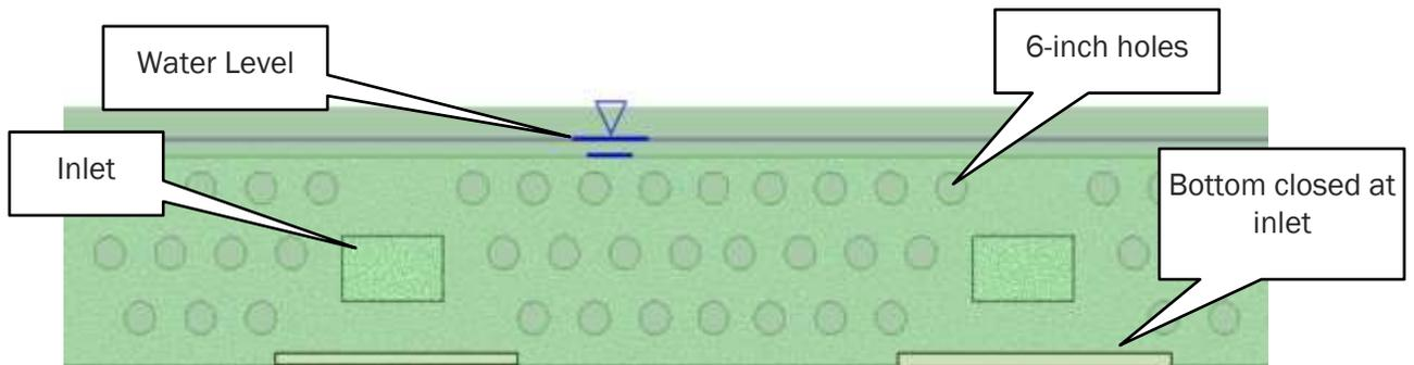
**Figure 4-5. Inlet baffle configuration used in 3D CFD model**
