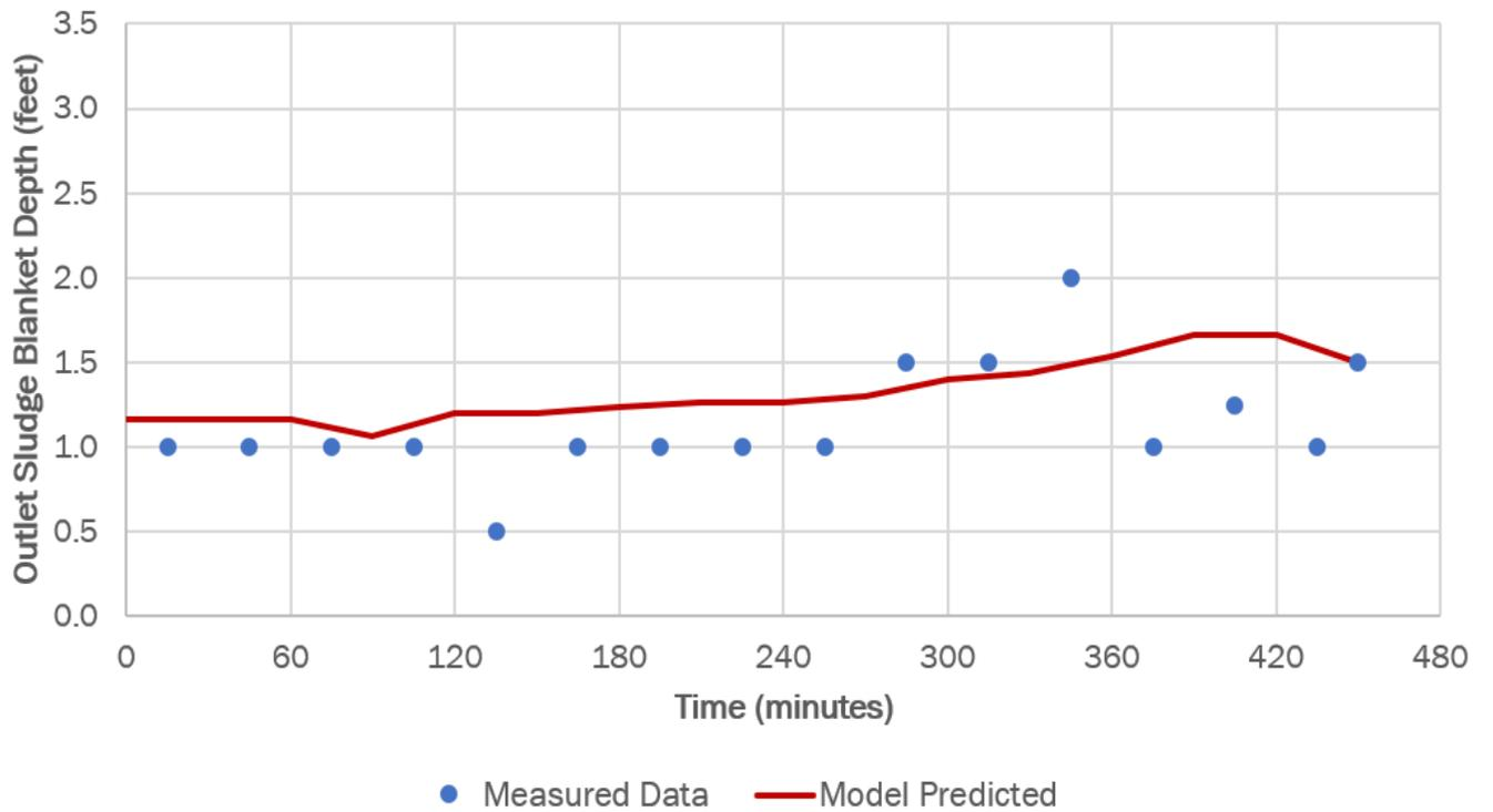
Figure 2-11. Primary Clarifier 2 measured and predicted SBD at outlet end
