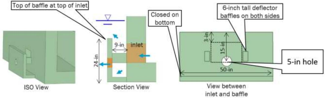
Figure ES-5. Recommended diffuser plate configuration
