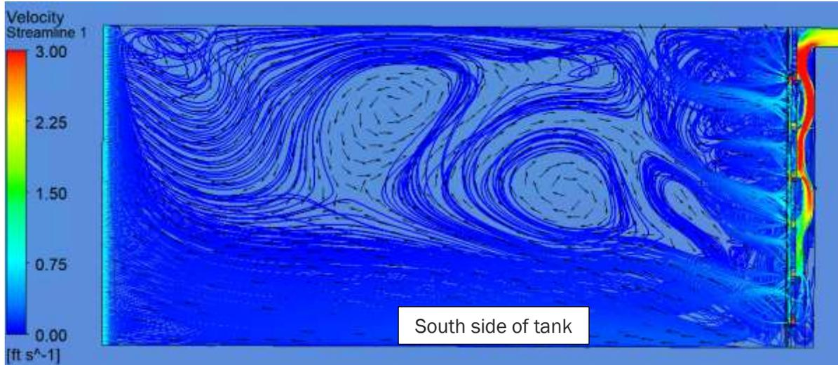
Figure 4-6. Primary Clarifier 2 inlet baffle model predicted stream lines – plan view
