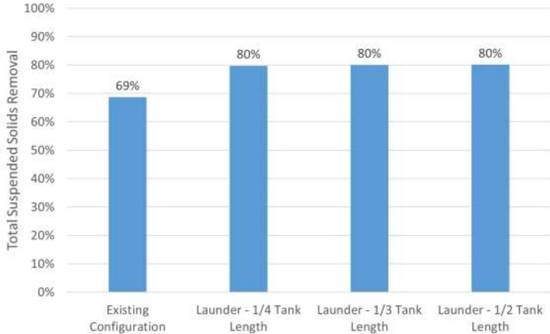
**Figure 3-3. Predicted TSS removal for various launder extension lengths**
