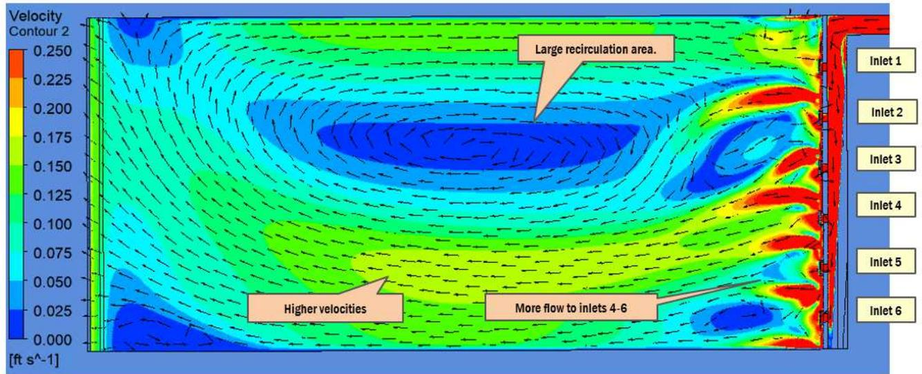
**Figure ES-4. Primary Clarifier 2 swirling action during peak flow conditions (SOR = 1,660 gal/ft<sup>2</sup>-d)**
