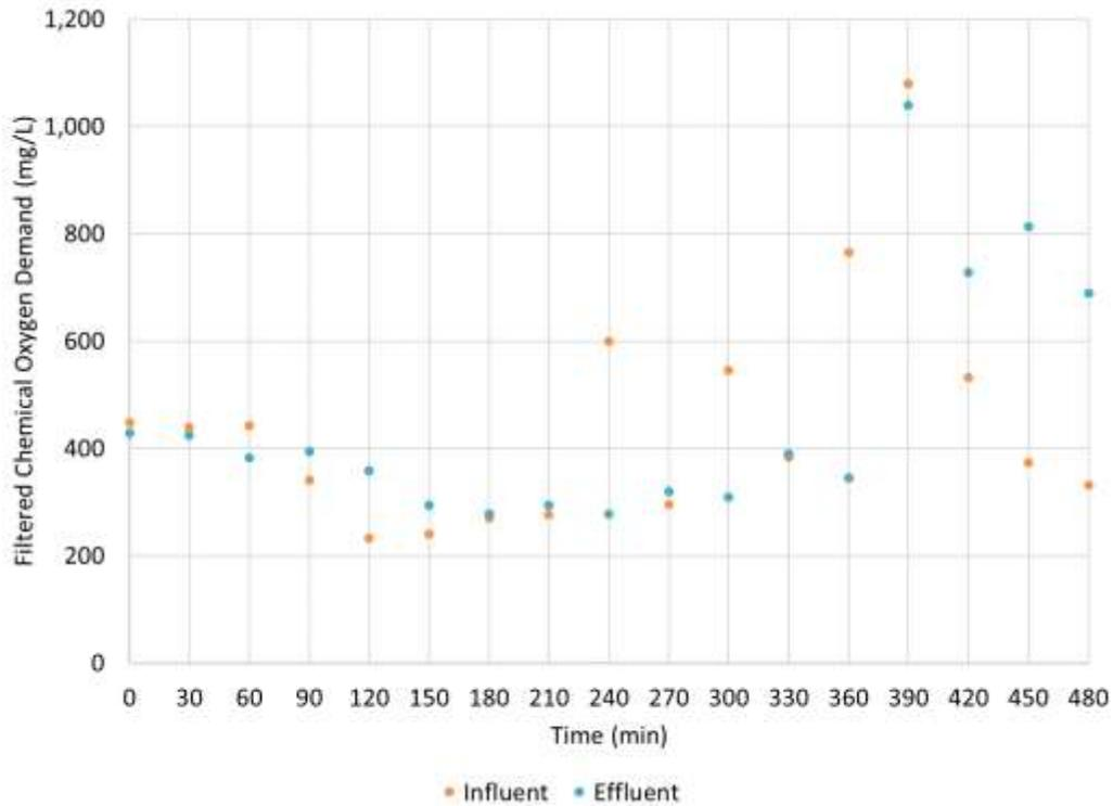
**Figure 5-2. Stress test Primary Clarifier 2 influent and effluent filtered COD**
