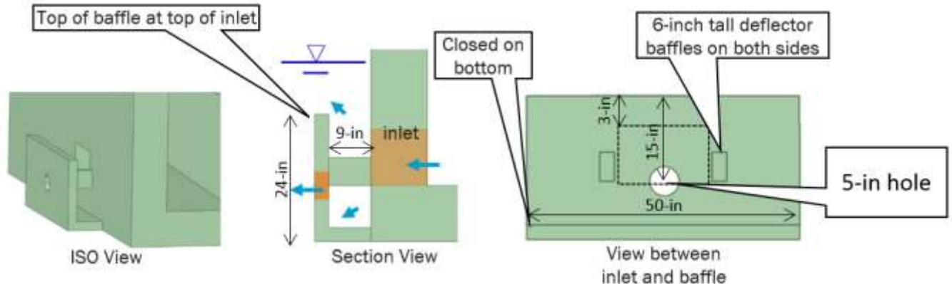
**Figure 4-13. Alternative 2 diffuser plate configuration**
