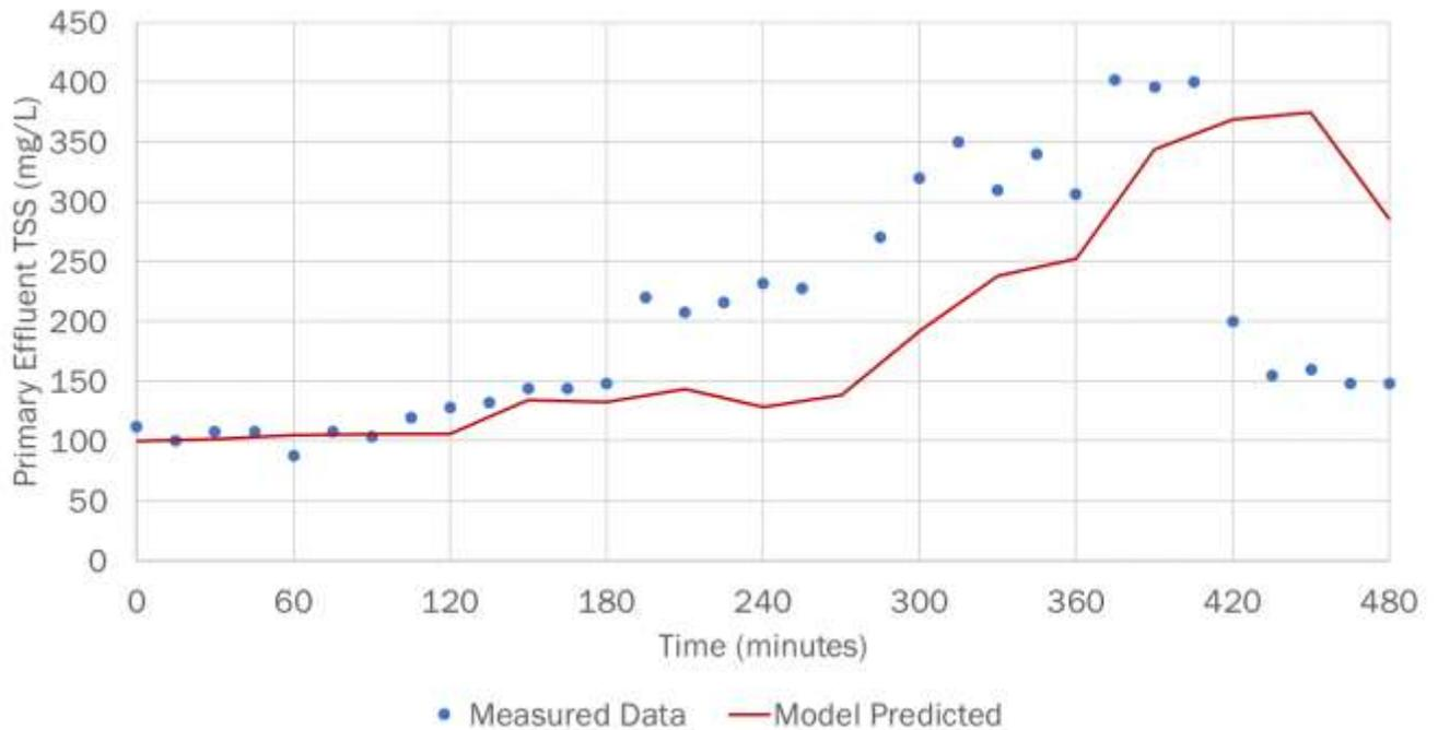
Figure 2-5. Primary Clarifier 2 measured and predicted PE TSS
