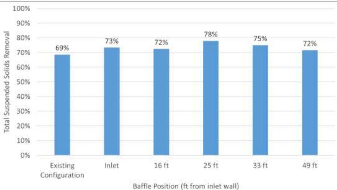
**Figure 3-5. Predicted TSS removal for various baffle locations**
