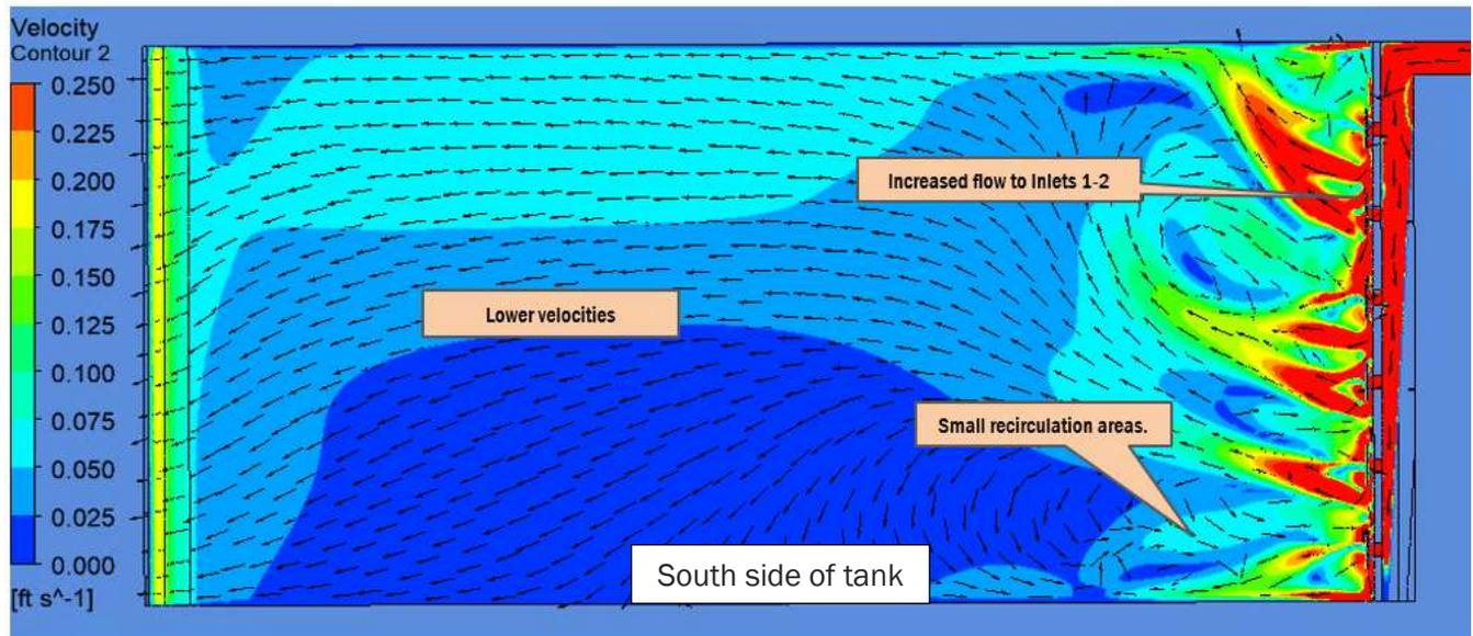
Figure 4-14. Primary Clarifier 2 diffuser plate Alternative 2 stream lines – plan view (includes inlet stub baffles)
