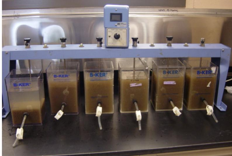
Figure 2-3. Flocculation Jar Test Apparatus
