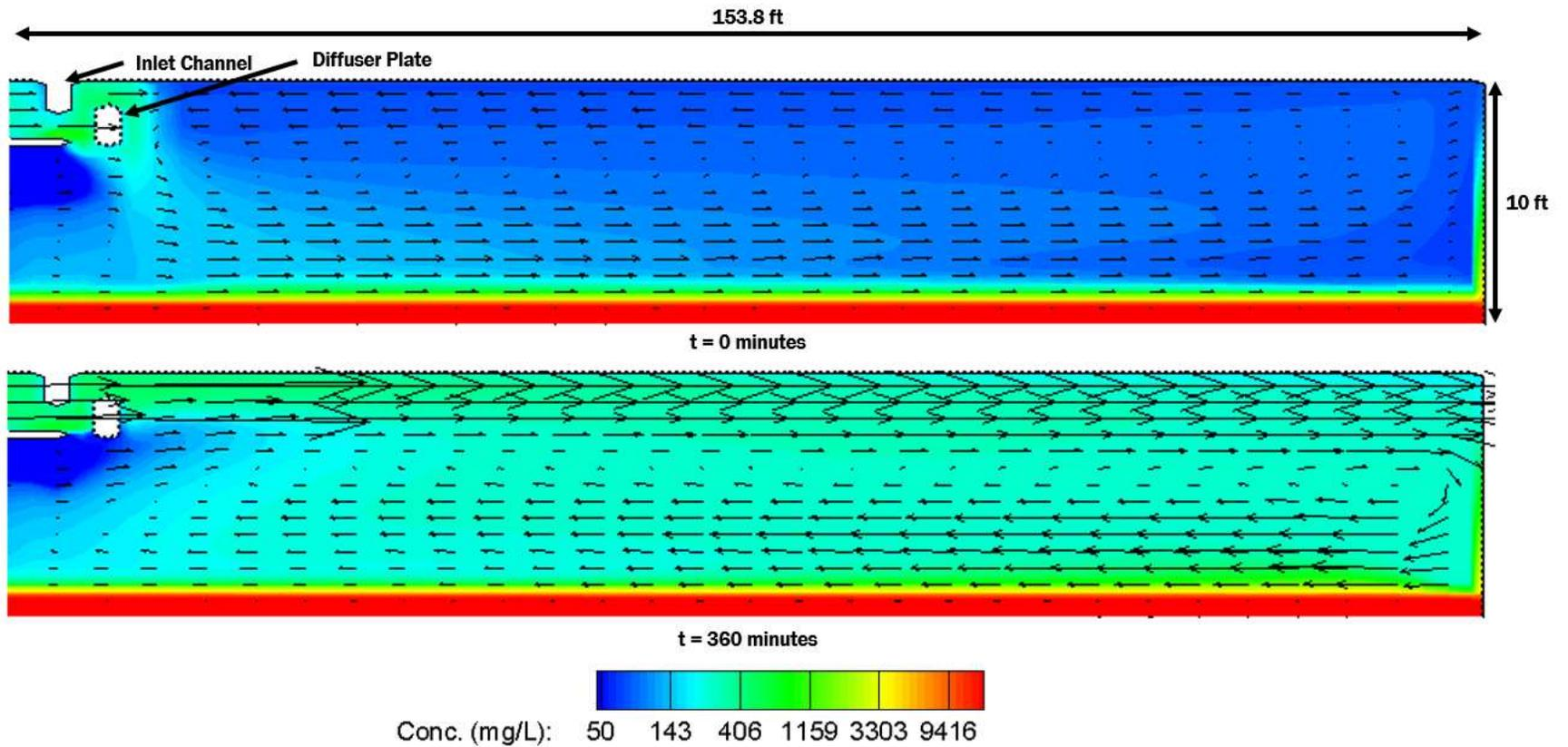
Figure 2-13. Primary clarifier 2 calibration at test time 0 and 360 minutes
