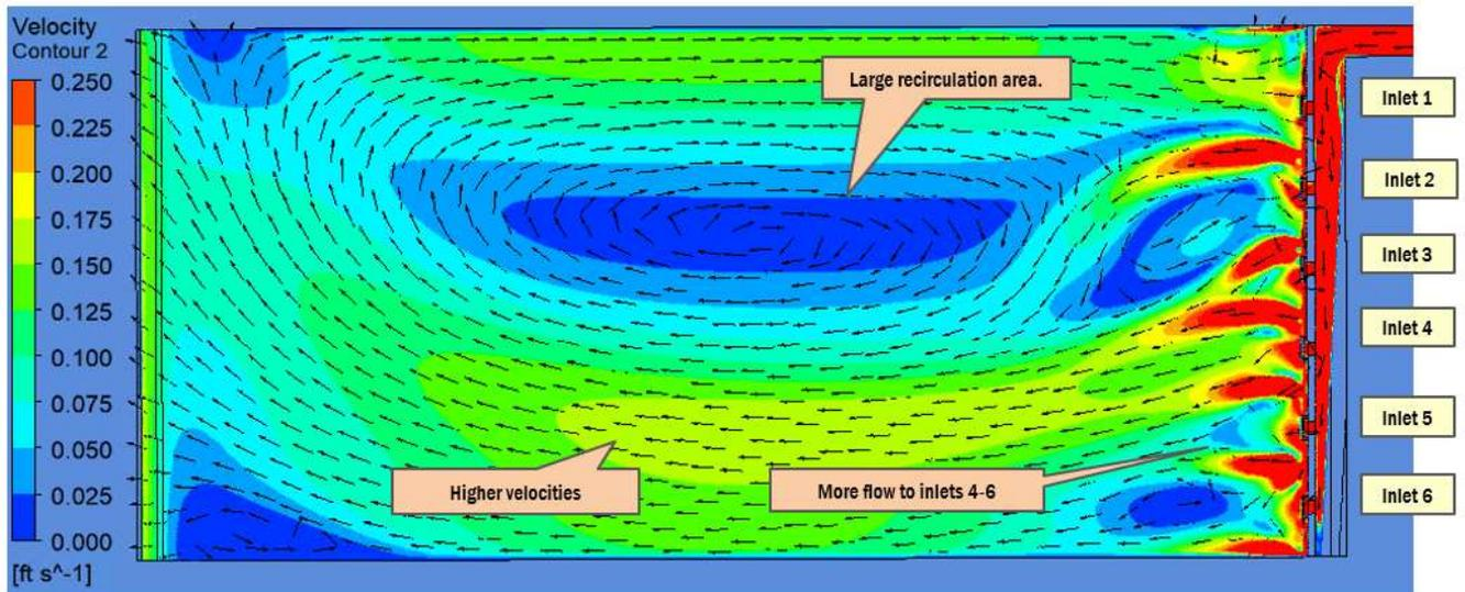
**Figure 4-1. Primary Clarifier 2 predicted swirling action during peak flow conditions**
