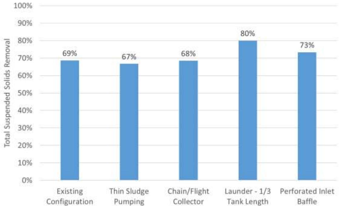
**Figure 3-2. Predicted TSS removal for various performance enhancement configurations**
