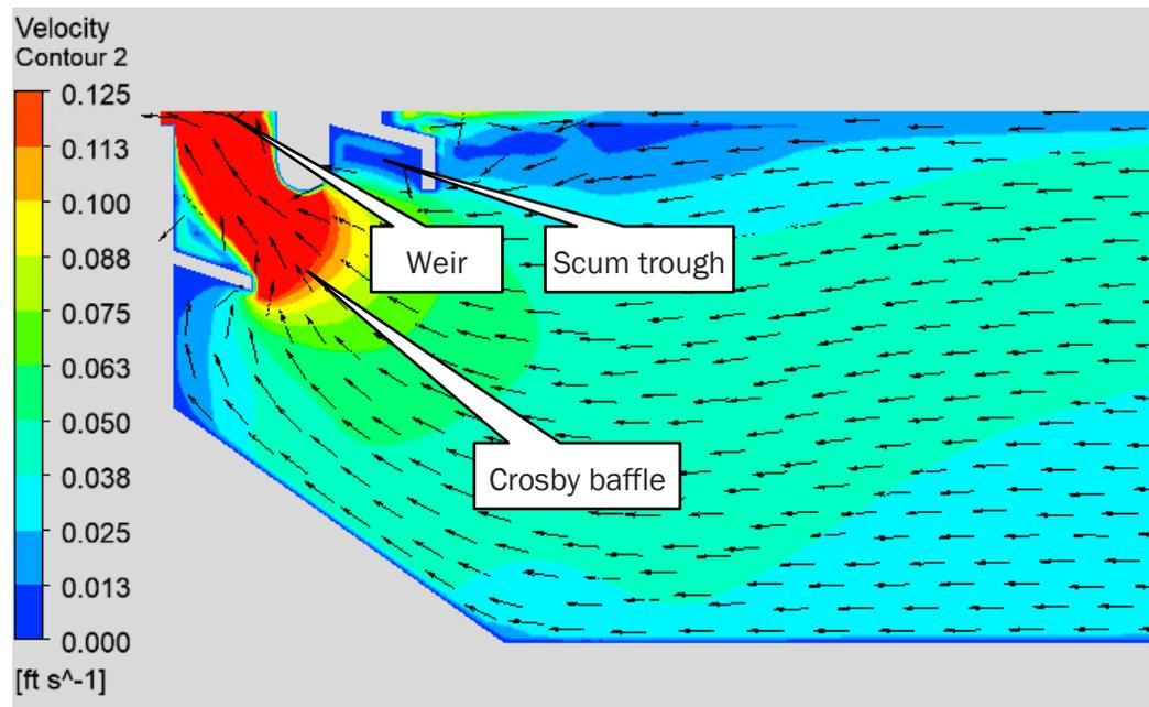
**Figure 4-17. Primary Clarifier 2 end wall with Crosby type baffle velocity profile – section view**
