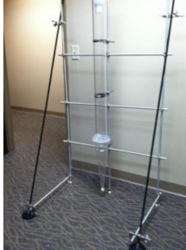
Figure 2-5. Discrete Settling Column
