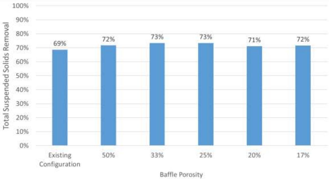
**Figure 3-4. Predicted TSS removal for various inlet baffle porosity**
