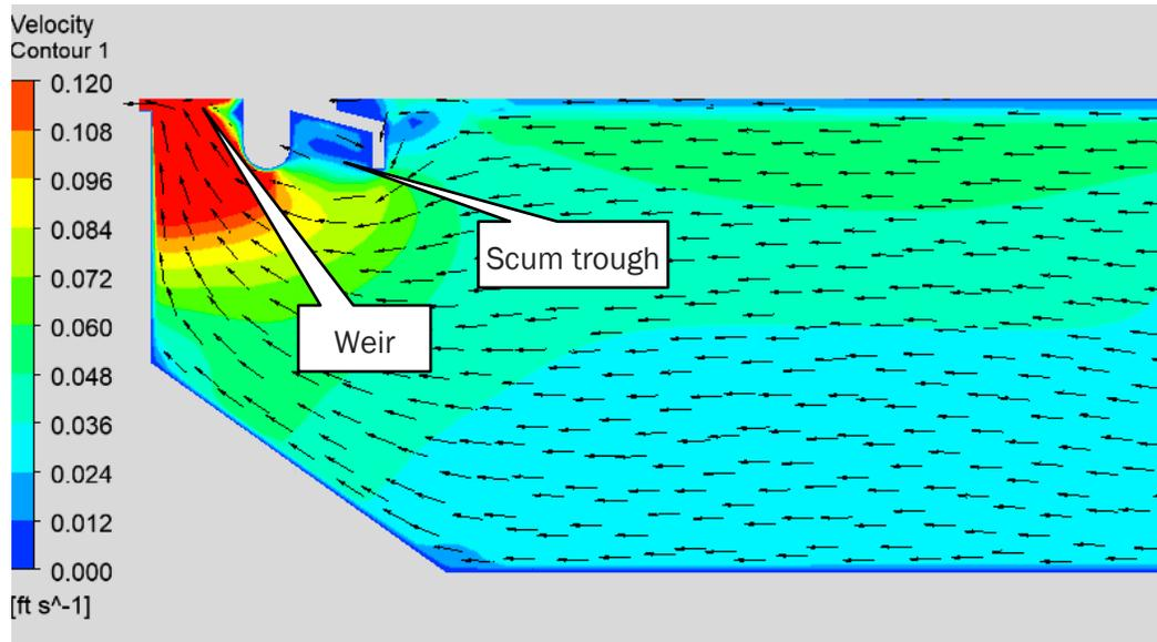
**Figure 4-16. Primary Clarifier 2 existing end wall configuration velocity profile – section view**
