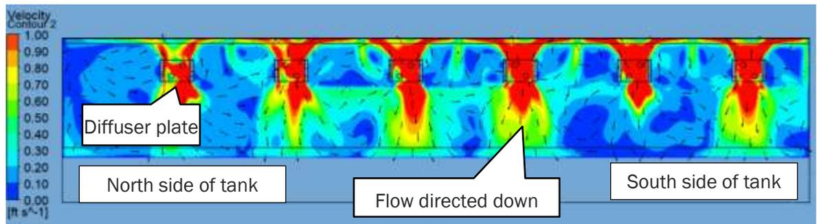
**Figure 4-12. Primary Clarifier 2 diffuser plate Alternative 1 stream lines – section view**
