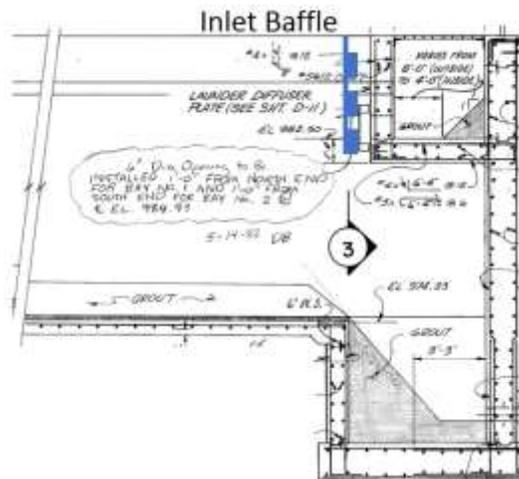
**Figure 3-8. Primary Clarifier 1 and 2 diffuser baffle**
