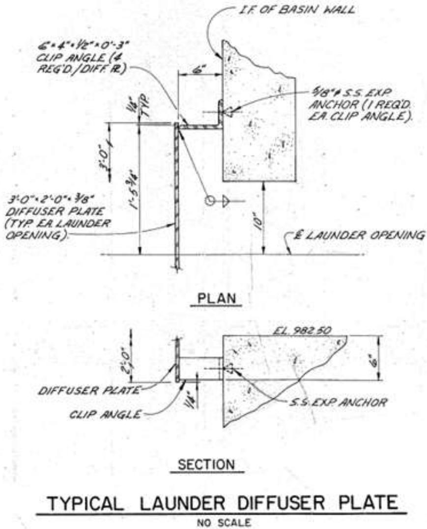
Figure 4-8. Existing diffuser plate details
