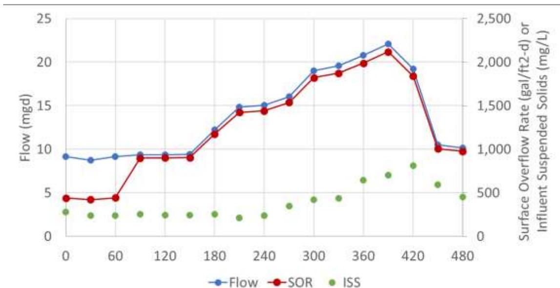
Figure 2-4. Primary Clarifier 2 stress test surface overflow rate and influent solids
