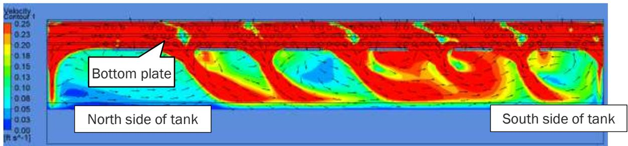
Figure 4-7. Primary Clarifier 2 inlet baffle model predicted stream lines – section view
