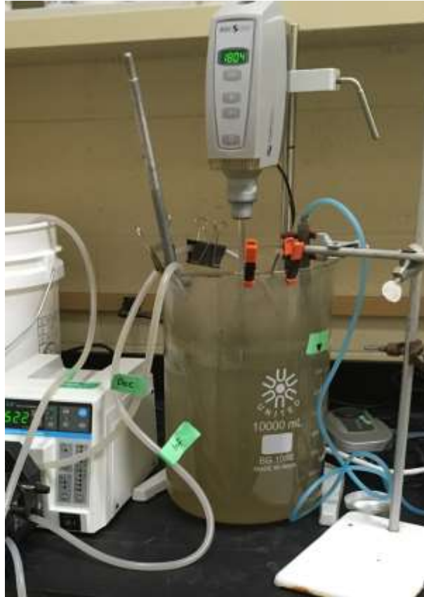
Figure 8. Washout Test Reactor on Day 3.
