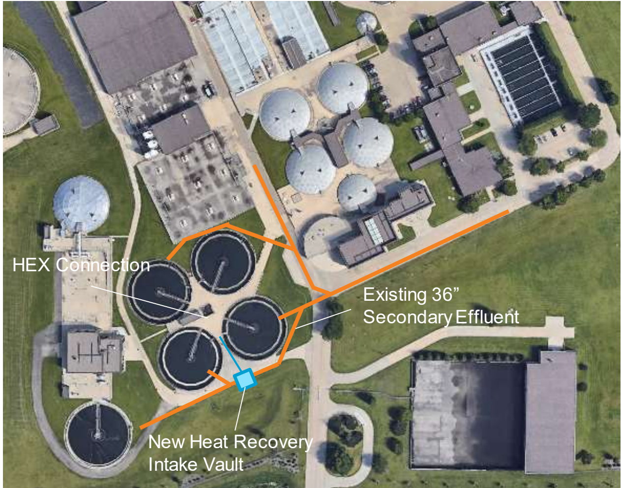
Figure 3-2. New heat recovery intake vault and piping
