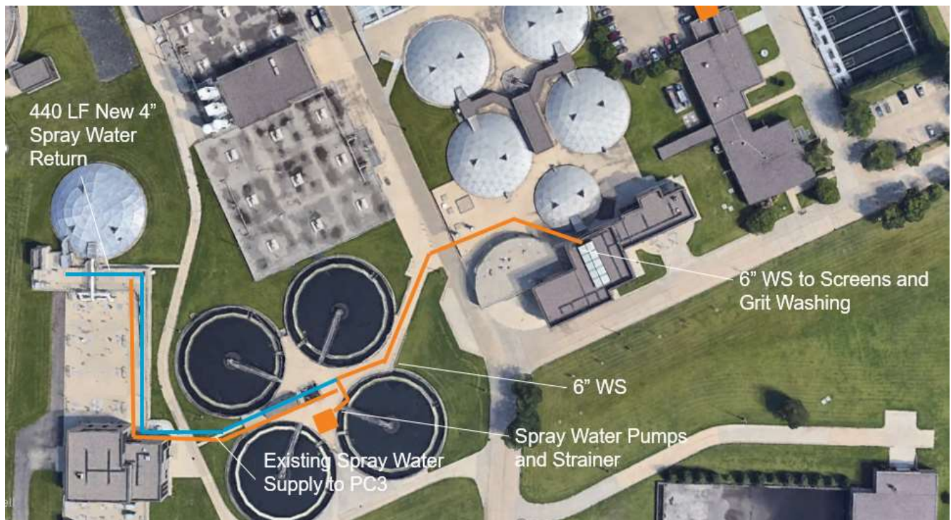
Figure 4-3. Piping to route effluent water from PC3 HVAC back to spray water
