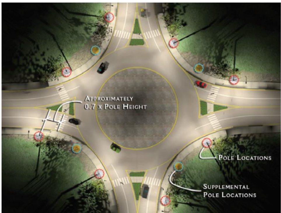
Figure 16: Typical Roundabout Placement of Lighting Units
